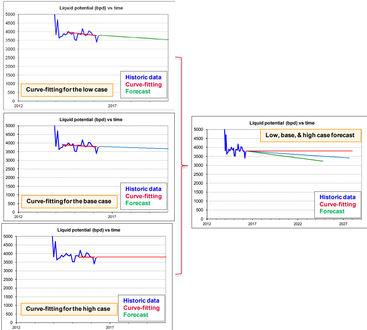
Figure 50: Selection of representative periods for the low, base and high estimate forecasts
