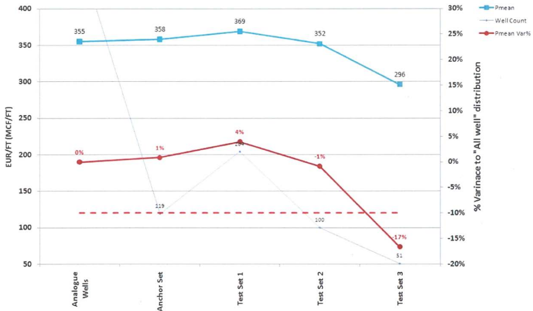
Figure 58: Well count, Mean and variance for Analogous wells, anchor wells and test wells
